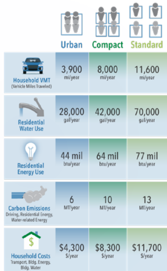
Figure 7: Comparison of Resource Consumption by Density Source: City of Cedar Rapids adapted from City of Denver, Colorado
